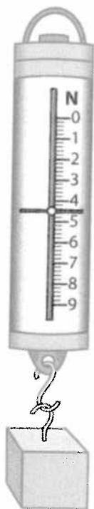
Figure 1-6. Spring scale: Force or weight is measured with a spring scale. This scale reads 4.5 N.
