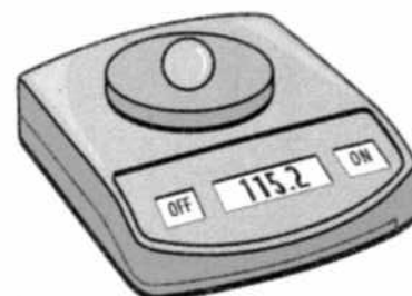
Figure 1-3. Electronic balance: The steel ball has a mass of 115.2 g.
