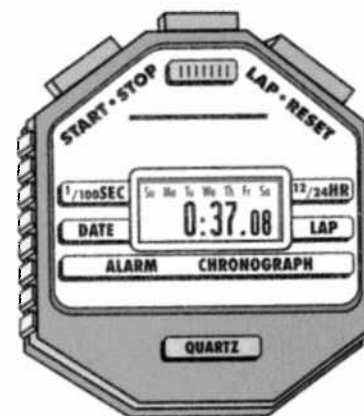
Figure 1-5. Stopwatch: Minutes are recorded to the left of the colon. Seconds (to the one-hundredth place) are recorded to the right of the colon. The elapsed time is 37.08 s.
